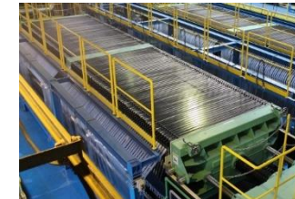
Chlor-alkali electrolyzer "Acilyzer™"
